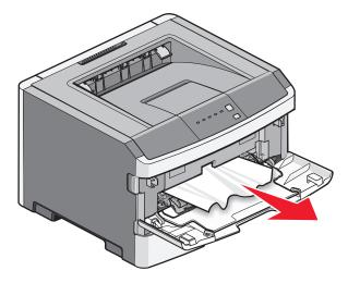
Paper jammed in the manual feeder can usually be grasped and pulled straight out. If the jam cannot be removed this way, check for jammed paper behind the photoconductor kit and toner cartridge unit. For more information, see "Clearing jams behind the photoconductor kit and toner cartridge" on page 99.
