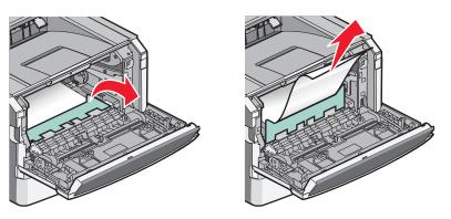
**Note:** If the paper is not easy to remove, then open the rear door to remove the paper.
