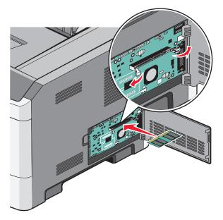
**6** Push the memory card into the connector until the latches *click* into place.
