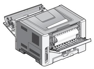
Clearing jams 105 **3** Remove the jammed paper.
