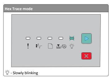
Make sure the printer is not in Hex Trace mode. If the "Hex Trace mode" light sequence appears, you must exit Hex Trace mode before you can print your job. To exit Hex Trace mode, turn the printer off and back on.
