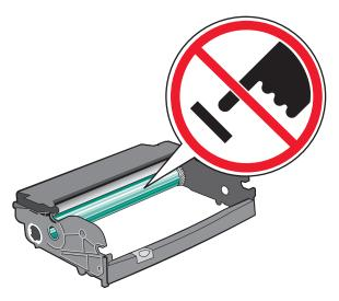
**5** Insert the toner cartridge into the photoconductor kit by aligning the rollers on the toner cartridge with the tracks. Push the toner cartridge in until it *clicks* into place.
